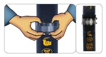
3. Slide the shield back over the gasket.
